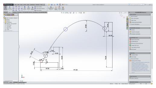
The final calculated Angle is 61.5, with a range down to 60.5 up to 62.0. And a forward and backwards driving range of +3.5 inches and -13.5 inches
